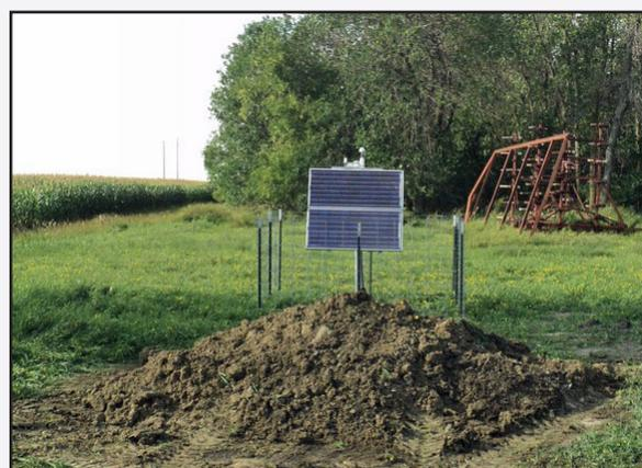
**Figure 2.** Seismic monitoring station located northwest of Fargo near Gardner, North Dakota shortly after installation. The seismometer is housed in a sealed circular vault just below ground level (buried beneath the excavated soils). The solar panel powering the instrument and supporting electronics is surrounded by protective fencing.
