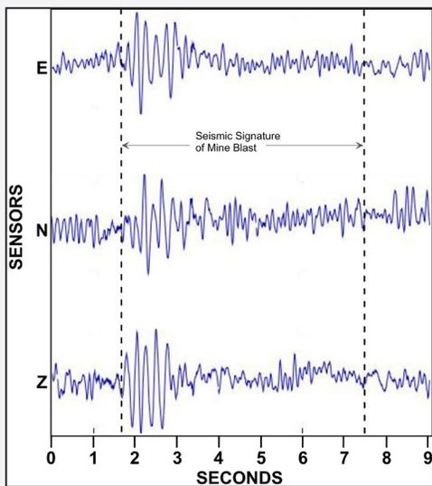
**Figure 6.** Seismogram from recent rock blasting at the Falkirk Mine in north-central North Dakota showing the characteristic seismic signature of a typical mining or quarry blast.
